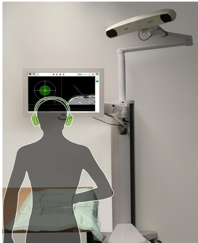
**Fig. 2** Test setup featuring navigation system with on-screen visualization and phantom with outline of typical user
